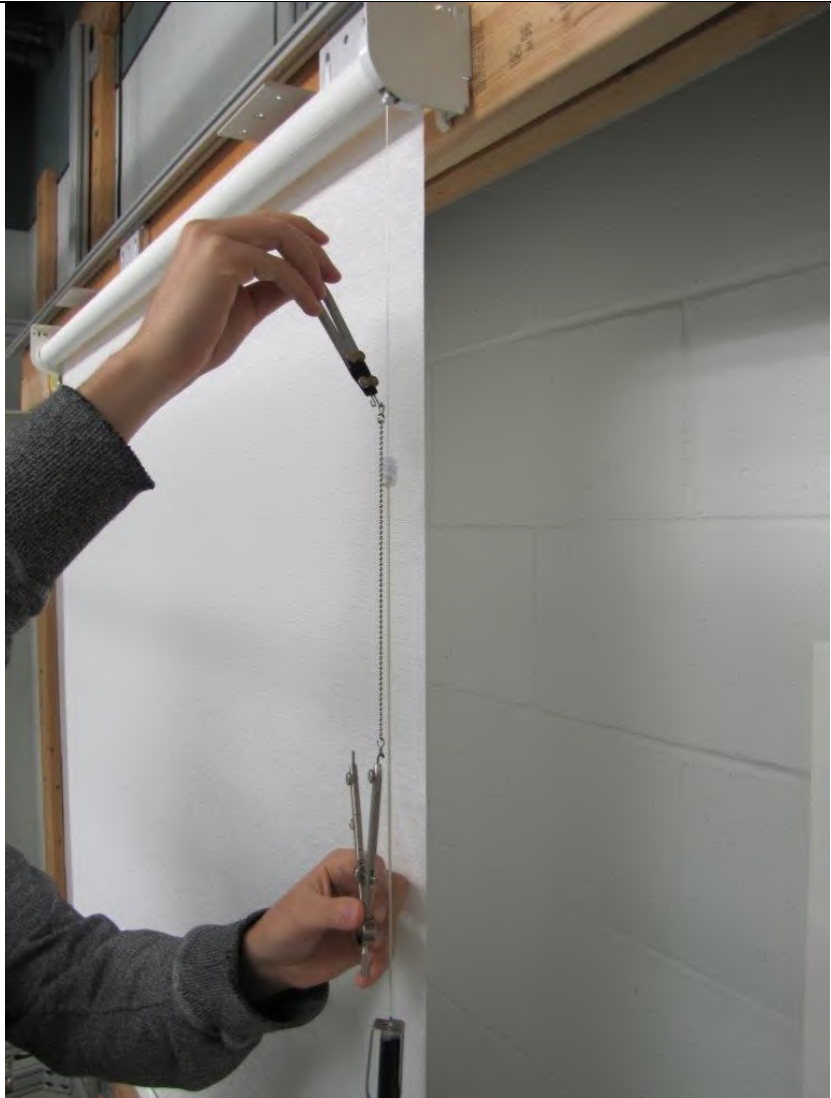
The analyst uses the cord length gauge to assess if the cord length is greater than 22 cm during load application.
